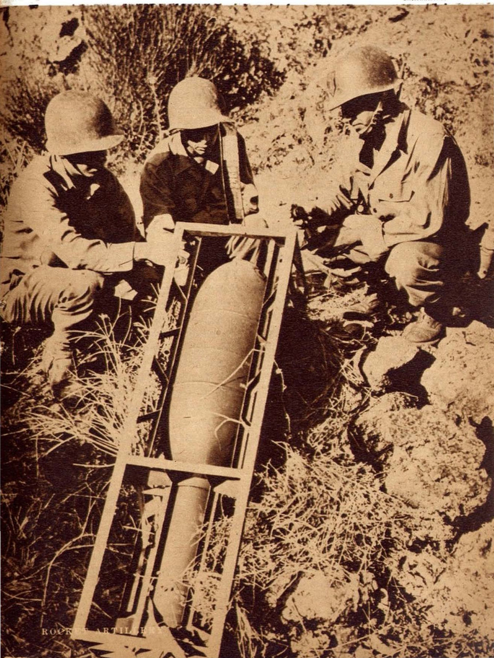
The 32 cm. German incendiary rocket is shipped in a special crate which serves as the launching rack, when the outer wrapping is removed.
